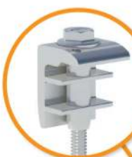
EFO™ The End Fastening Object secures XR Rail® ends, fitting 30-40mm module heights.
