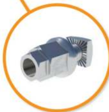
Bonded Attachments The bonding bolt attaches and bonds the L-Foot to the rail. It installs with the same socket as the rest of the system.
